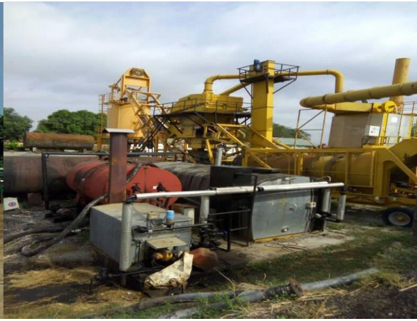
70/80 TPH ASPHALT PLANT WITH HOT AND COLD FACILITY
