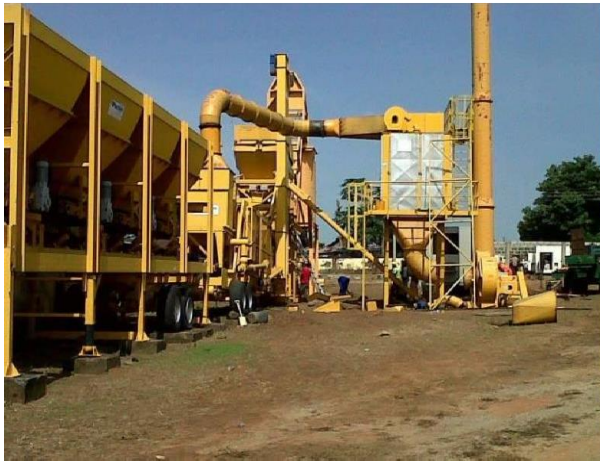
70/80 TPH ASPHALT PLANT WITH HOT AND COLD FACILITY
